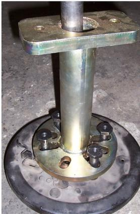
3. Place the GGT-600 over the axle and attach to the backing plate / bearing hub, using the special nuts supplied. No need to remove the shrink ring.
